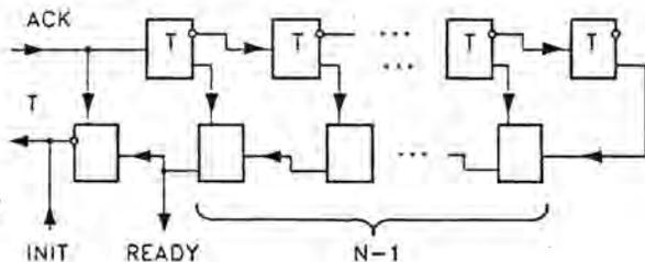
Fig.8. Controller.  $T$  - asynchronous  $T$  flip-flop; the leftmost cell is RSFQ inverter.
