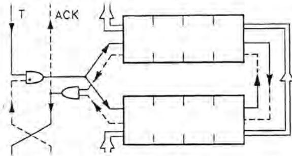
Fig.7. N-cell FIFO register contains two shift registers - one with timing flow along, and one counter data flow.
