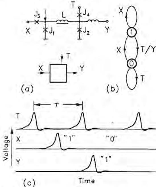
Fig.1. D flip-flop as simplest "logic" RSFQ element: (a) notation and equivalent circuit; (b) diagram of state transitions induced by SFQ input pulses X and T. One followed by the output is marked with /Y; (c) time diagram.
