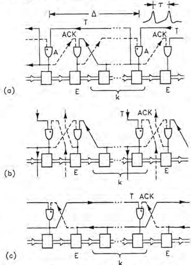
Fig.6. Shift structures buffered with cells E. The timing (T) pulses flow: (a) counter; (b) across and (c) along the data (—) pulses.
