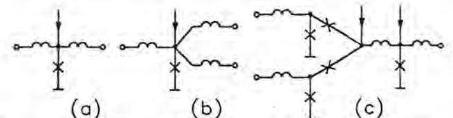
Fig. 4. Interconnecting elements: (a) one stage of JDTL; (b) split buffer; (c) confluence buffer.
