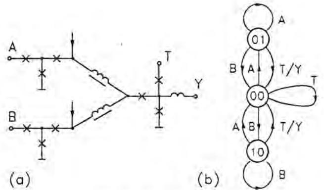
Fig.2. Exclusive OR clocked flip-flop: (a) equivalent circuit; (b) diagram of state transitions induced by input pulses A, B and T. Ones followed by the output is marked with /Y.
