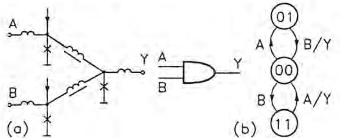
Fig.3. Coincidence junction or Muller C-element: (a) notation and equivalent circuit; (b) diagram of state transitions induced by SFQ input pulses A and B.
