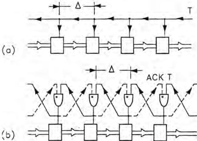
Fig.5. Simplest data shift structures: (a) externally clocked shift register; (b) self-timed shift register.
