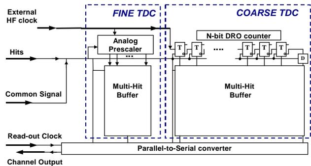
Fig. 2. A single channel of the multi-hit TDC, showing the coarse and fine components, as well as the I/O and control channels.
