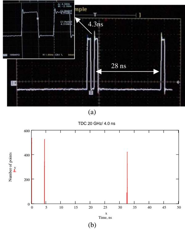
Fig. 5. (a) Hit pattern generated using HP-8000 observed on a Tektronix oscilloscope. (b) Histogram obtained from the measured data using the VXI data acquisition software shows the correct time between hits.
