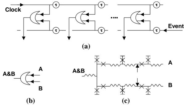
Fig. 4. (a) The dynamic AND prescaler uses anti-parallel pulse propagation. The time vernier is connected to dynamic AND gates. The symbol and schematic for this novel gate are shown respectively in (b) and (c).
