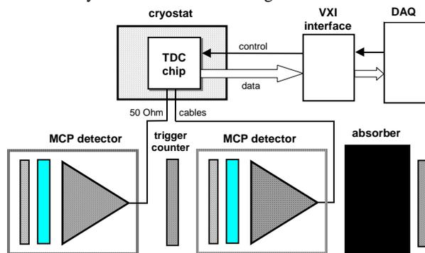
Fig. 1. Block diagram of the prototype TOF system. In this design, cosmic ray muons trigger micro-channel plate (MCP) detectors providing the start and stop events for the superconductive TDC chip.
