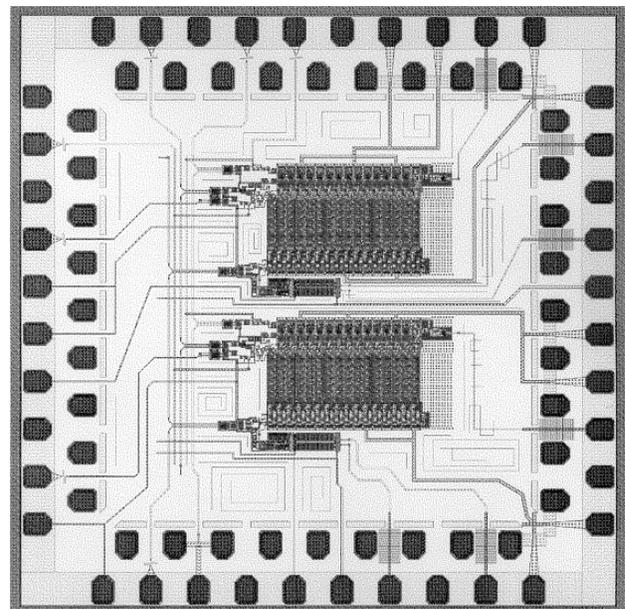
Fig. 3. Two-channel digital multi-hit TDC
