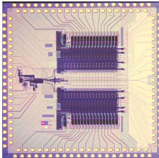
Fig. 3. Microphotograph of a single-channel All-Digital Receiver (ADR) chip based on the first-order low-pass delta ADC, digital in-phase and quadrature (I&Q) mixer, and decimation digital filters. This 1 x 1 cm<sup>2</sup> chip consists of ~12,000 JJs and dissipates ~3.5 mW.
