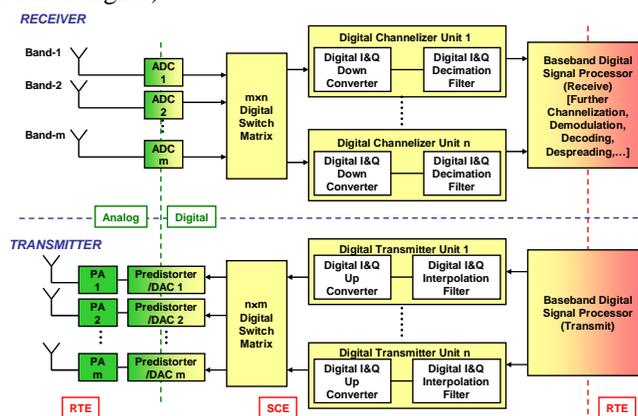
Fig. 1 Block diagram of Digital-RF Transceiver using combination of room-temperature electronics (RTE) and cryogenic superconductor electronics (SCE) elements located on different temperature stages of a cryocooler.
