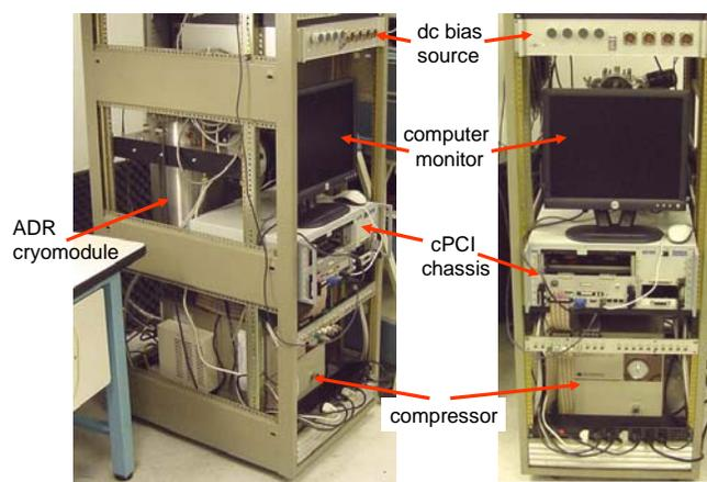
Fig. 4 Photo of the cryopackaged ADR test setup using commercial Sumitomo cryocooler mounted into the lower part of standard 19-inch rack.
