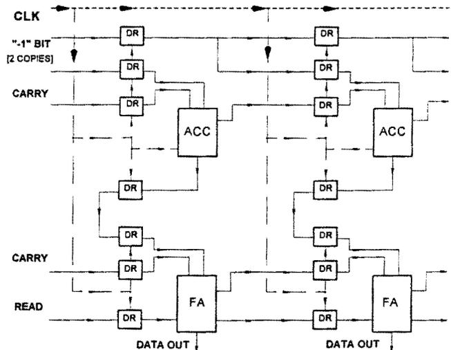
Fig. 2 Block diagram of a 2-bit fragment of the decimation digital filter for a 20 GHz operation.
