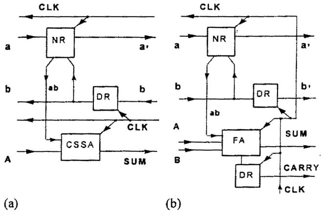
Fig. 1 Block diagrams of single-bit modules of (a) serial multiplier; (b) parallel multiplier (PMM).
