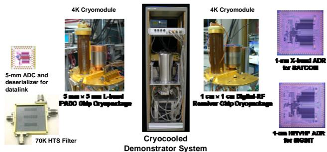
Fig. 3. Rack-mounted cryocooled Digital-RF receiver system (center) and its main replaceable 4K cryomodules for  $5 \times 5 \text{ mm}^2$  (left) and  $10 \times 10 \text{ mm}^2$  chips (right). The HTS analog filters are mounted on a 70K stage.
