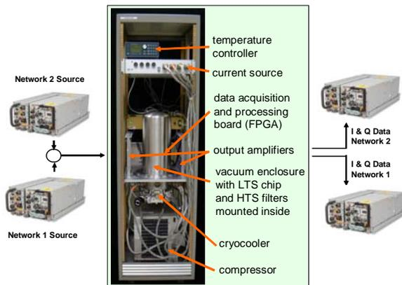
Fig. 4. The multinet datalink system. The  $ht^2$  Digital-RF receiver system is based on 70K HTS analog filter and 4K RSFQ wide-band L-band ADC and deserializer, and 300K FPGA processor. Two hopping networks were simultaneously received, dehopped, and demodulated.
