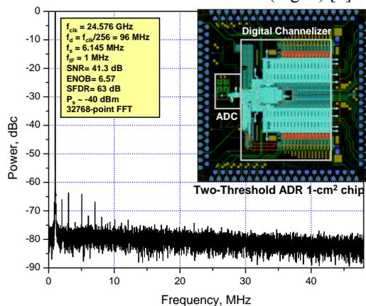
Fig. 2. One half of the digitized spectrum (from one digital filter) of a two-threshold receiver (ADR) chip. The output I and Q data rates are 96 MSample/s corresponding to decimation ratio of 256.
