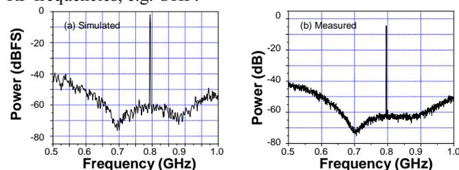
Fig. 1. Two-implicit-loop ADC: (a) Simulated and (b) measured spectra of  $\Delta\Sigma$  modulator used to digitize a 200 MHz band around 800 MHz. The 5-mm ADC chip included a 1:16 deserializer and was clocked at 10.24 GHz. The input signal frequency is 796 MHz. The measured SNR is 31.6 dB in 660-915 MHz band.
