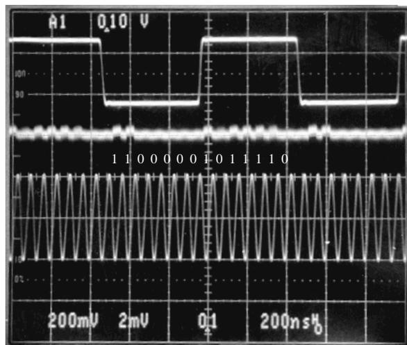
Fig. 4. Correct high-speed operation of a single-channel 14-bit TDC measuring the period between event pulses. Traces from top to bottom are: event signal, output data, and upload clock. The measured time between event pulses is 12,382 clock pulses at reference frequency 12.382 GHz (the event signal frequency was 1 MHz).
