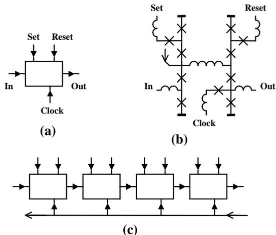
Fig. 2. A novel design of a parallel-to-serial converter: (a) Notation of a single cell. (b) Schematics of a single cell. (c) Block diagram of a parallel-to-serial converter.
