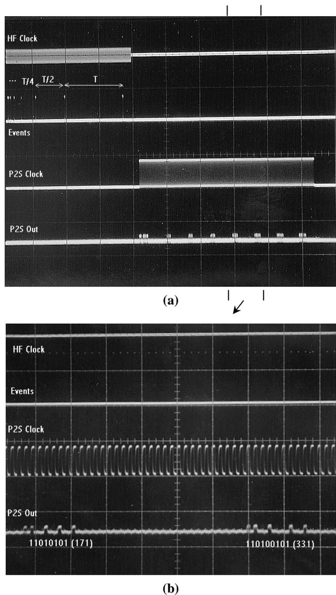
Fig. 3. Successful operation of a 30-bit, 8-word multi-hit TDC. (a) Measurement of the time between successive event pulses. (b) Zoom-in of two successive counts. Traces from top to bottom: HF clock, events, parallel-to-serial converter clock, and output.
