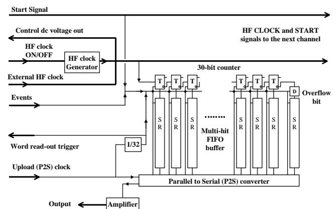
Fig. 1. Block diagram of a single channel of multi-hit TDC.
