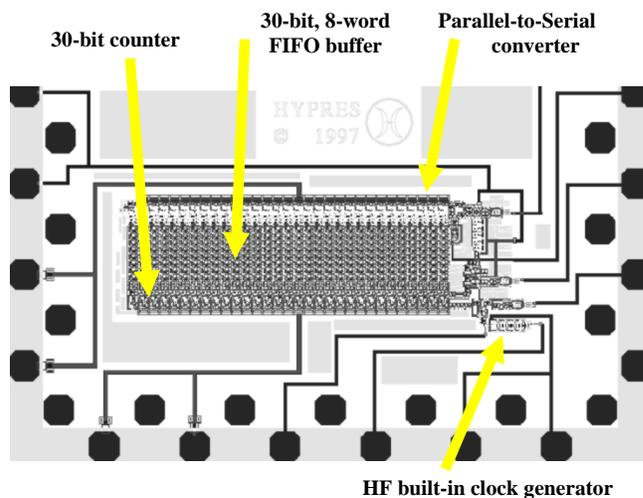
Fig. 3. Layout of a 30-bit, 8-word multi-hit TDC circuit. Chip size is  $5 \text{ mm} \times 5 \text{ mm}$ .
