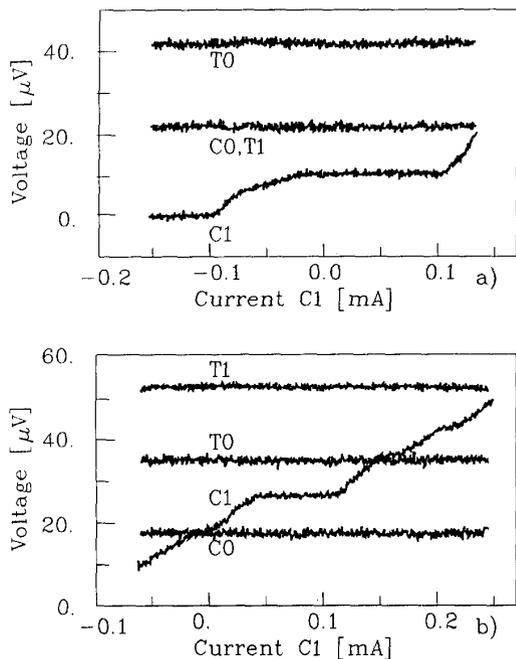
Figure 4. Experimentally measured DC voltages of two-bit reversible binary counter on the inputs  $T_0$ ,  $T_1$  and on the carry outputs  $C_0$ ,  $C_1$  of BIT0, BIT1 as function of current applied to  $C_1$  for regimes of adding (a), diminishing (b).
