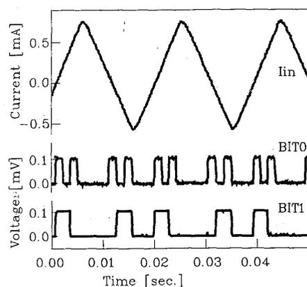
Figure 5. Measured digital outputs  $V_0$ ,  $V_1$  of two-bit A/D converter in response of input signal current  $I_{in}$ .
