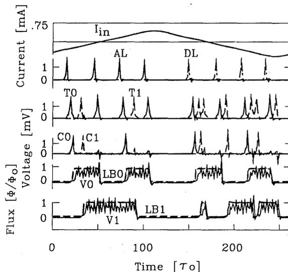
Figure 3. Results of numerical simulation of the circuit shown in Fig.1b for experimental parameter values:  $I_{C1} = I_{C2} = 1/2 I_{C3} = 1/2 I_{C4} = 2/3 I_{C5} = 2/3 I_{C6} = 1/2 I_{C7} = 1/2 I_{C8} = 1/2 I_{C9} = 1/2 I_{C11} = 2/3 I_{C10} = 2/3 I_{C12} = I_{C13} = I_{C14} = 0.125$  mA,  $L1 = 2$   $L2 = 2.4$   $L3 = 12$   $L4 = 16$  pH,  $V_C = 0.3$  mV,  $\beta_C = 1$ ,  $\tau_0 = 3$  ps,  $R = 0.2$  Ohm.
