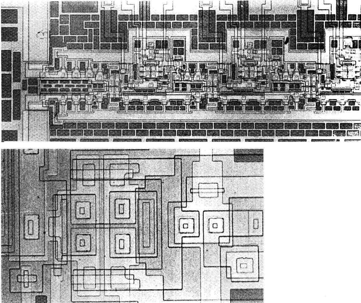
Figure 2. Microphotographs of 8-bit A/D converter chip.
