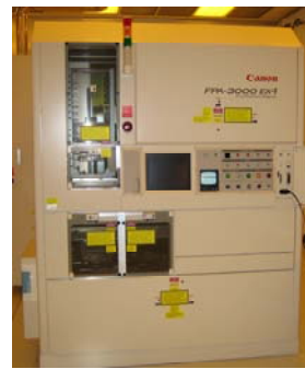
Fig. 1. The new HYPRES photolithography: Cannon EX-4 stepper.
